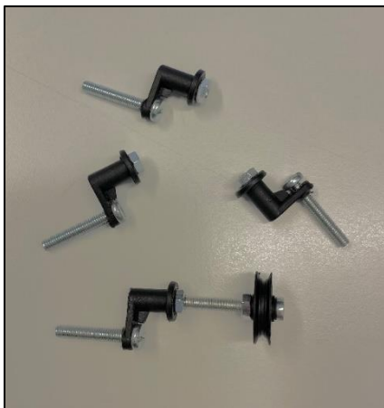
Figure 13: solution for the crank* and belt drive
