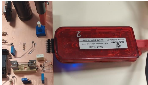
Figure 32 : Branchement Pickit3
