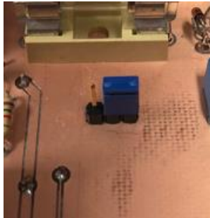
Figure 31 : Position cavalier alimentation USB
